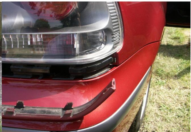
Pictures 4 & 5. The bumper can be easily removed without removing this trim, but it certainly helps to have it off when refitting so that you can see that the bumper locates correctly onto the two runners on each side.
