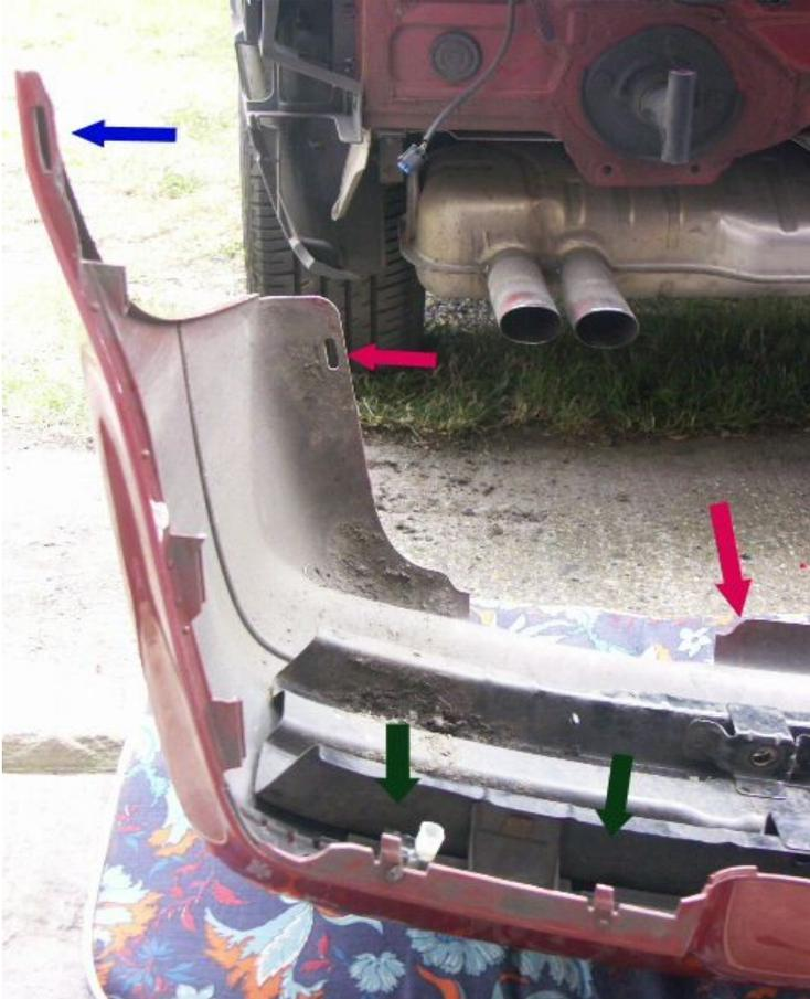
The trick, having removed those bolts and studs, is getting the bumper to slide back. And be warned, when it does slide back it does so suddenly and drops off the back of the car, but don't worry, it won't hit the ground. It's fall will be abruptly halted by the cables to the parking sensors. NOT what you want. Either have a helper or position something to prevent the bumper falling off.
