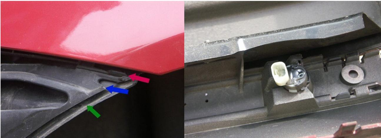
Once the bumper is off the sensors can easily be removed by firmly pressing the moulding to one side and popping the sensor up from below. The sensors cannot simply be metered out to tell if they are good or bad as they seem to have capacitance or inductive elements.
