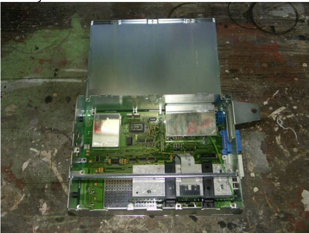
Picture 5. Once levered off from the mounting bracket the unit can easily be prised open. As you can see there's no user serviceable parts inside. And due to the nature of the construction the only plug is very unlikely to work loose.
